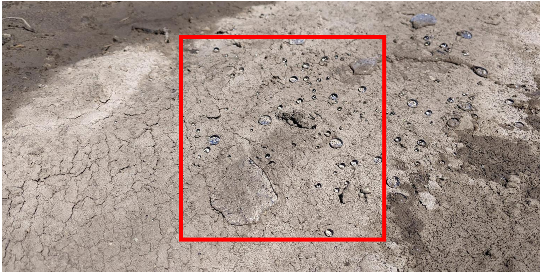
Water “beads” on treated surface
