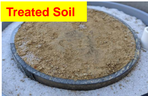
No heave due to frost action
