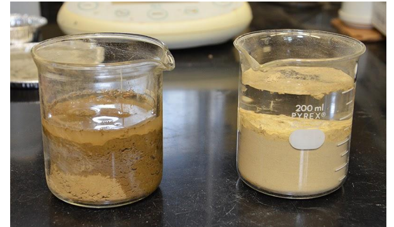
Water permeates the untreated soil in the left beaker, while water in the right beaker stays on top of the OS treated soil.
