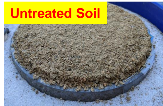
Measured heaving of ~6mm
