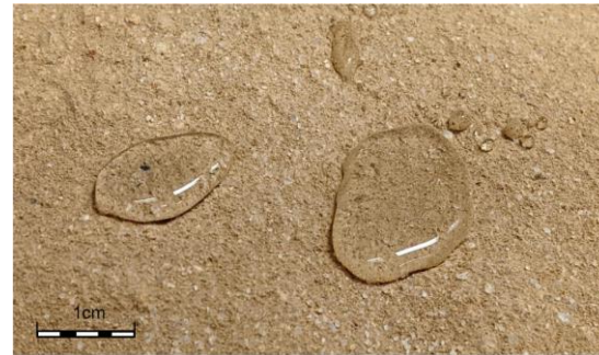
Water “beads” on the treated surface
